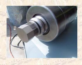
The tube expander is designed to be used with our standard hydraulic power pack. The tool is manually placed on the tube end and actuated by means of a foot switch. The expander's stroke is easily adjusted to achieve the exact required expanded diameter. The tool steel expanding collets will expand most common tube materials including copper, aluminum, steel and stainless steel.
